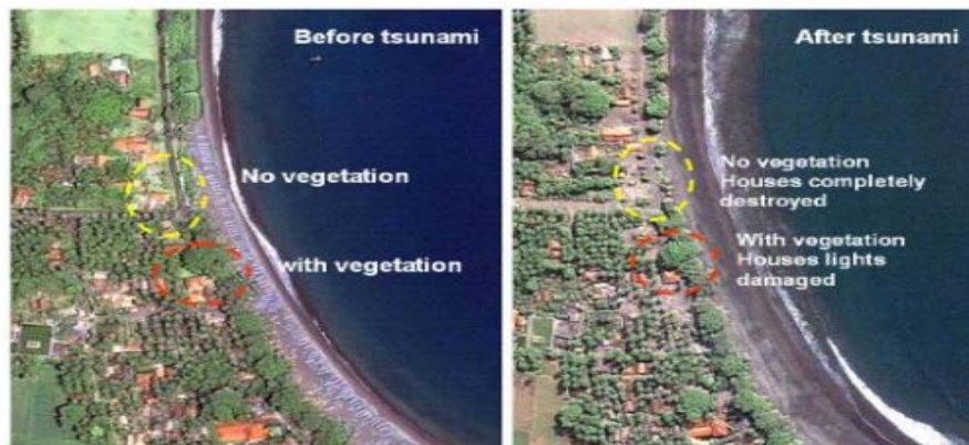
Plate 1.5 Ikonos imagery before and after the 2006 West Java tsunami shows how vegetation reduced tsunami impact at Pangandaran Beach (source: CRPS www.crips.nus.edu.sg/ )
